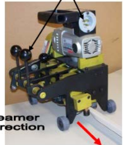
Seamer Locked on the Adjacent Seam
