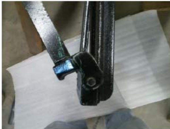
Open Crimping Jaw of the QuadLok Crimper
