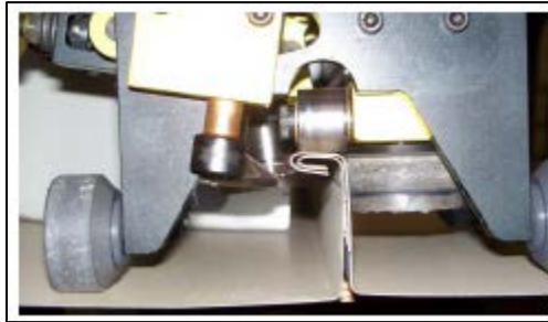
Note the Orientation of the Seamer and Locking Handles
