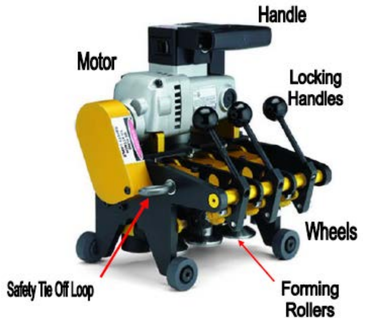
Primary Seamer Produces a TripleLok Seam
