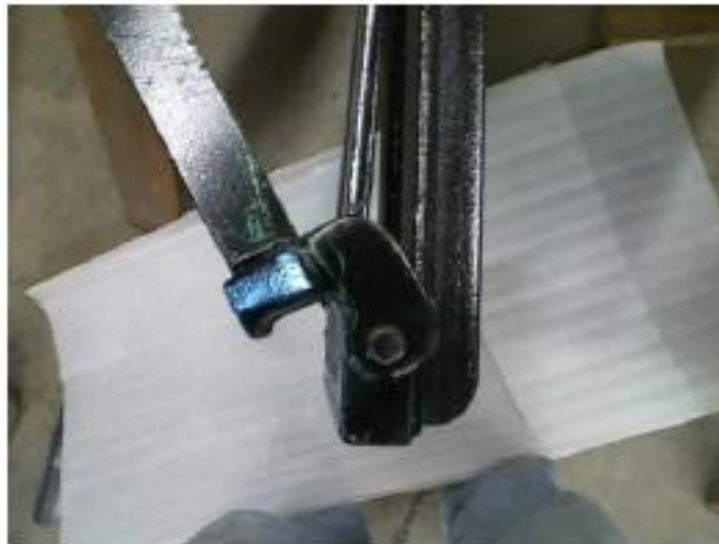
Open Crimping Jaw of the QuadLok Crimper
