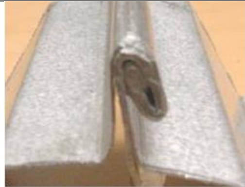
Finished QuadLok Seam
